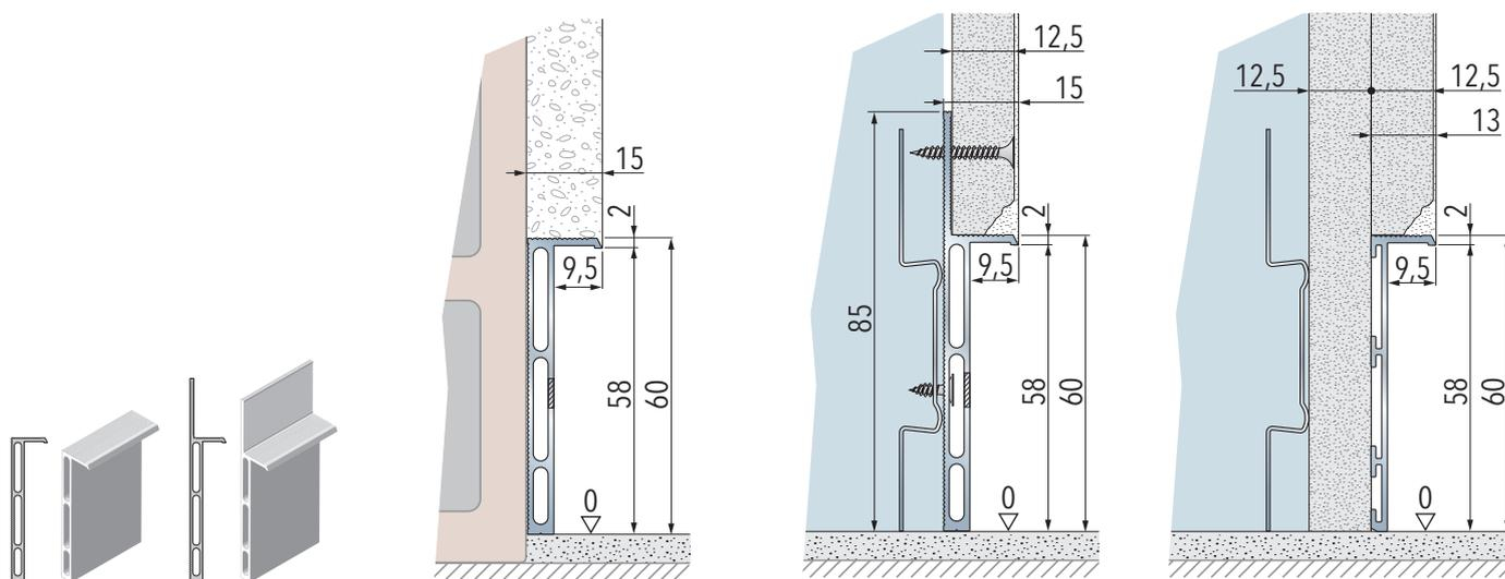
The aluminium profile is supplied in 2000 mm long bars. Useful space in height for the baseboard: 58 mm
