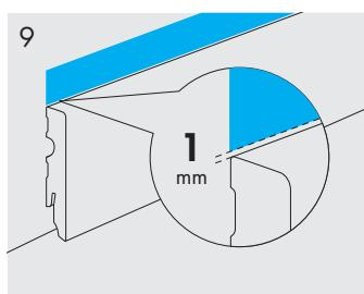
Apply painter's tape to the wall, about 1 mm above the installed skirting board.
