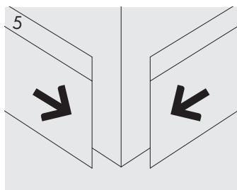
Glue the skirting boards in the outer corner to the wall, press against the wall, leave to dry.
