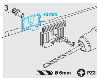
Drill a hole in the wall, connect the clip to the spacer and screw the clip to the wall using a screw.
