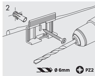
Drill a hole in the wall and screw the clip to the wall with a screw.
