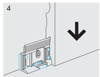
Put the skirting board onto the clip from above and press down firmly.
