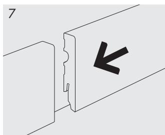
Glue the skirting board sections to the wall, press against the wall, leave to dry.
