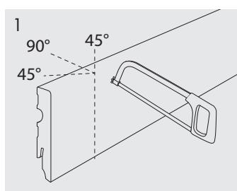
Cut the skirting board at 45° (corners) or 90° (joints).
