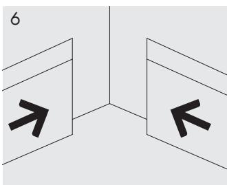
Glue the skirting boards in the inner corner to the wall, press against the wall, leave to dry.
