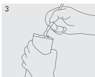
Impregnate the cut surfaces with finishing paint and leave to dry.
